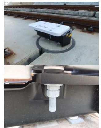
Automatic Train Stop (ATS)
